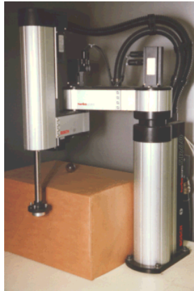
A Selective Compliant Articulated Robot Arm (SCARA).
