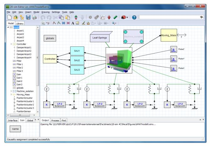
Figure 3: Model of the active vibration controller.
