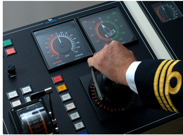
Figure 3: Assembly of ship bridge equipment with propulsion control units.
