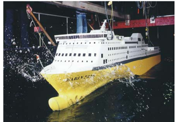
A ship model running in waves.
