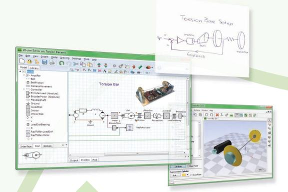
The sketch in converted into a model by dragging and dropping library blocks.
